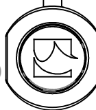
Detail 1:1 bottom rail round hembar 1 1/8" (Ø30mm) cable guided
